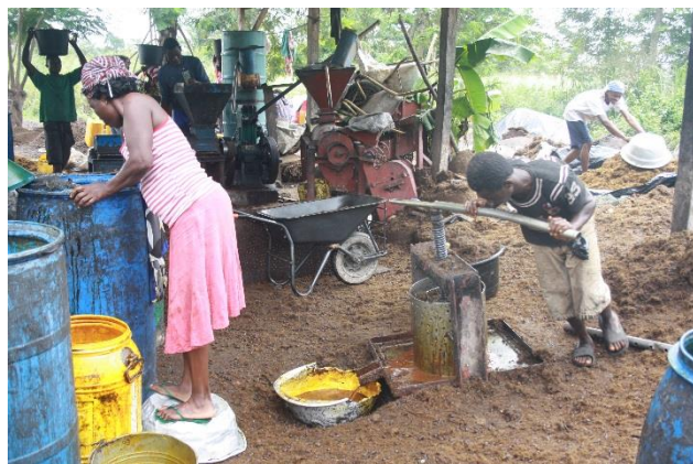
Plate 6. A palm oil mill in Assin Foso, showing threshing of fruit following first pressing to produce light oil (background), second pressing by hand to produce red oil (foreground) and storage of oil in barrels, each of which sells for ~ 600 Cedis (~£110).
